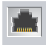
1000Base-T Gigabit Ethernet Port
